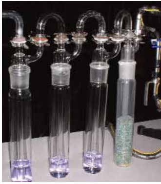
Figure 2. A typical set of impingers, which stand about 18 in. The first three are shown containing water and the fourth with granular silica gel to completely dry the sample gas. The impingers are immersed in an ice-water bath during sampling.
